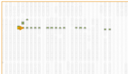
Use estimated position and slope at track end to extrapolate in opposite direction
